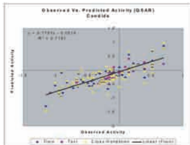
Fitness plot: This plot shows the significance of model predictive ability both in terms of explaining the variation in the activity as well as prediction of molecules in external test set.
